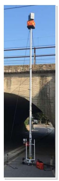
Kangur-Lift system is a telescopic column made of anodized aluminum with pneumatic extensions by hand pump, complete with manual locks that allow to stop the column at the desired height, with maximum height of 6.00 meters.
