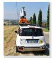
Level-Plane 16 is a static multi-axis platform created for automatic (non dynamic) leveling to ensure total verticality of the equipment with accuracy of +/- **30**" (or +/-**3**" with manual control) in all vehicle inclination conditions.
