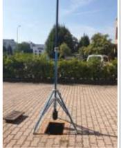
AD-EL Additional element of 1mt to be used only with Leica BLK360 laser scanner
