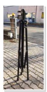
Upside down tripod is a telescopic lifter made of painted steel, with mechanical cranck system
